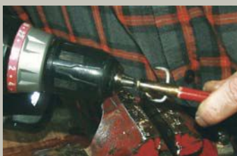
FIGURE 8: Bend nail ends to create barbs.
