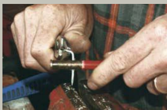
FIGURE 9: Use small drill bit to create a pilot hole for cap screw, drilling through primer-pocket hole.
