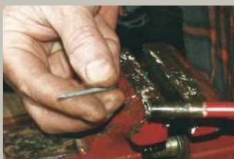
FIGURE 6: Sharpen both ends of standard finish nail.
