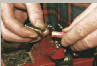
FIGURE 4: Slip prepared casing over shaft end and snug to end.
