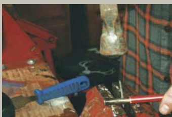
FIGURE 7: Gently tap finish nail through cross hole.
