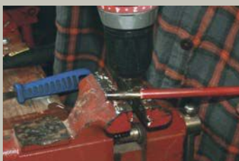
FIGURE 5: Drill hole across shaft using drill bit, resulting in extra-tight fit of finish nail.
