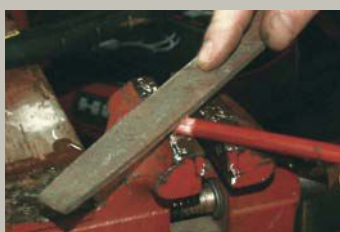
FIGURE 3: File shaft to accommodate .38 casing while also retaining a tight fit.
