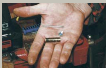
FIGURE 1: Weigh .38 Special (or .357 Magnum) casing, finish nail sharpened at both ends and small cap screw to achieve desired finished weight.
