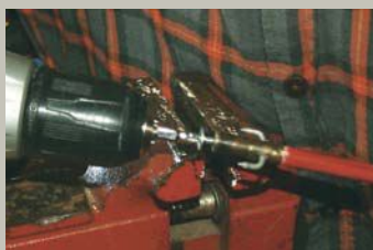
FIGURE 10: Carefully insert thin-thread, large-cap screw to secure casing and create tougher front face.
